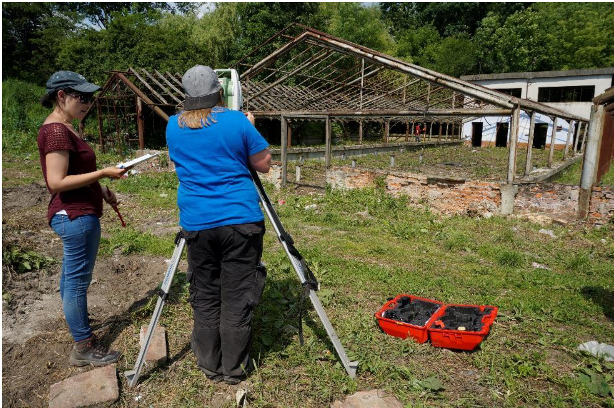
Figure 5: Measured topographic survey at the northern mass grave site using an Electronic Distance Measurer or Total Station (Copyright: Centre of Archaeology, Staffordshire University: Photograph courtesy of Jay Osborn)
