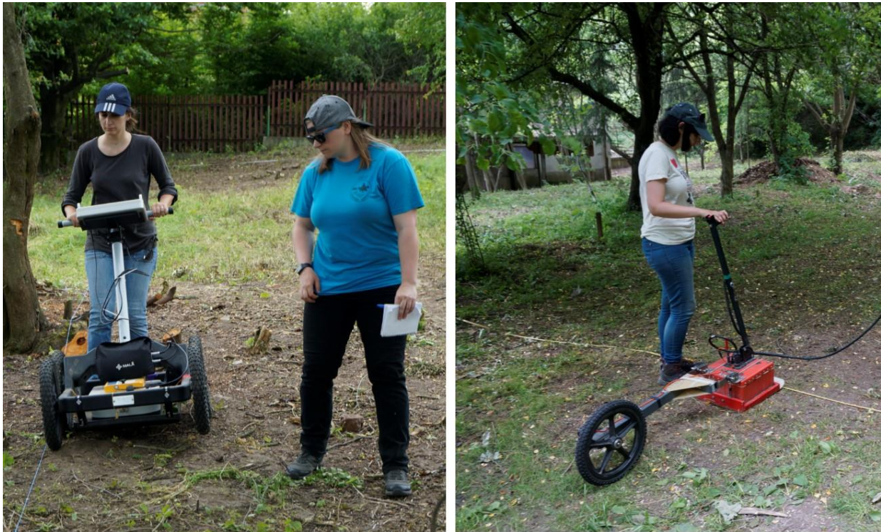
Figure 6: GPR systems used to complete the surveys at Rohatyn. The Mala Ground Explorer is on the left and the GSSI SIR 3000 system is on the right (Copyright: Centre of Archaeology, Staffordshire University: Photograph courtesy of Jay Osborn)
